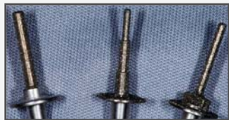
Figure 1: Available CEREC diamond milling tools for cutting the internal aspect of any restoration (from left to right): 1.6mm diameter; step bur 0.9mm diameter at tip; 1.2mm diameter.
