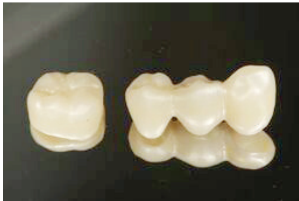
Fig. 5: Photo of the IPS e.max ZirCAD Multi after sintering.
