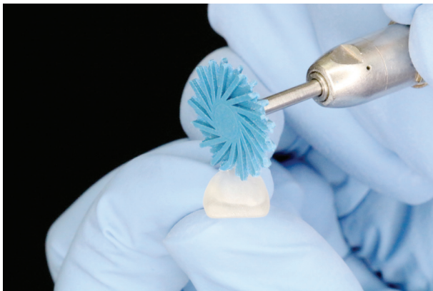
Fig. 19: The Coarse Twister and Blue Medium Twister were used to pre-polish the ceramic.
