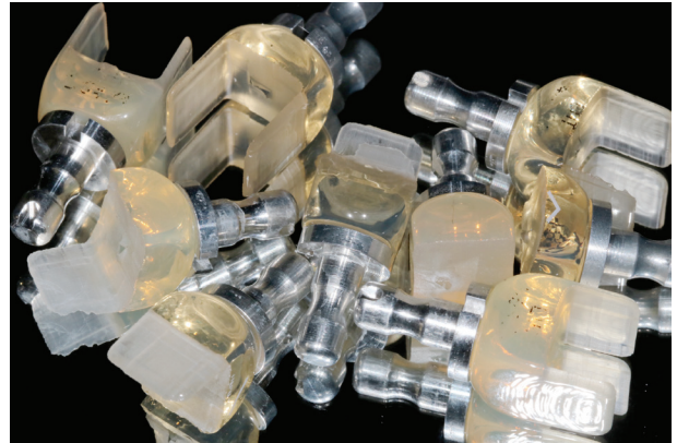
Fig. 16: On average, a single restoration took about six minutes to mill.
